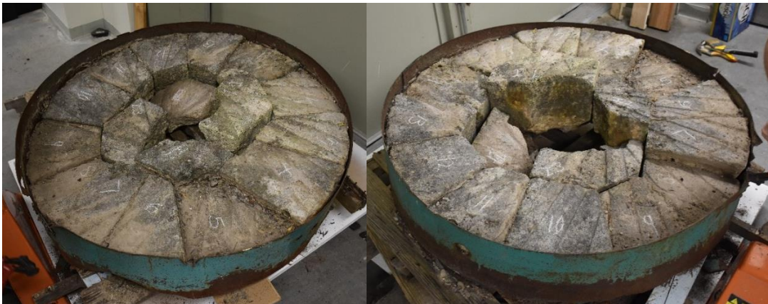
Different views of millstone with original ring. Note the stones had begun to shift.
